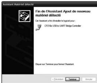
Img. 12: Successful installation of the second driver
